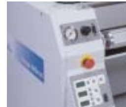
Fully integrated control panel for single location control of speed, pressure, temperature and roller positioning
